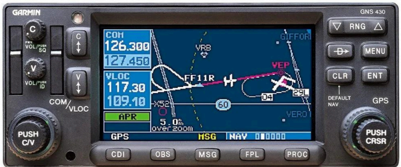
GARMIN 430 Global Positioning System (GPS) - WAAS Enabled
